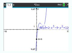
The result **Y=-3** should be displayed within the coordinate of the point (at the bottom right of the screen).
